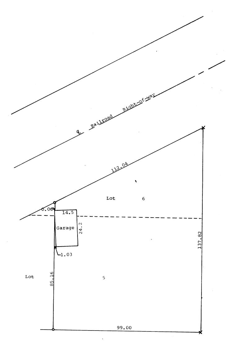
Scale - 1' = 20'• = Iron Pipe x = Cross in Concrete
